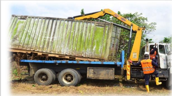
Transportation of abandoned caravan from the EEPSP site to the dump site using the self-loader
